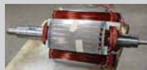
Completed rotor ready for the epoxy dip
