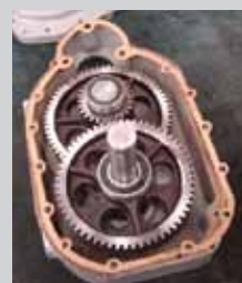
Gearcase with helical gears
