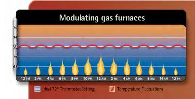
The Luxaire<sup>®</sup> Acclimate<sup>™</sup> modulating gas furnace has been designed to maintain your ideal temperature by modulating heating level in .50 or .65% increments. Comfort is dramatically increased as the furnace adjusts its level of operation up or down to offset the rate at which heat leaves your home.
